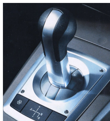
Manual Transmission Automatically Shifted (MTA)
